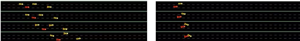
Figure 13: An individualized scenario selection result in Section 4.2.3. On the **left** is one scenario selected for normal AV models, and on the **right** is one scenario selected for AV models with left front perception defects. It can be observed that in the scenario on the right, the BV in left front of the AV is significantly closer and more aggressive.
