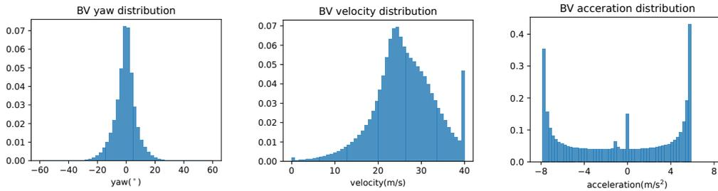
Figure 7: The yaw, velocity and acceleration distribution of BVs.
