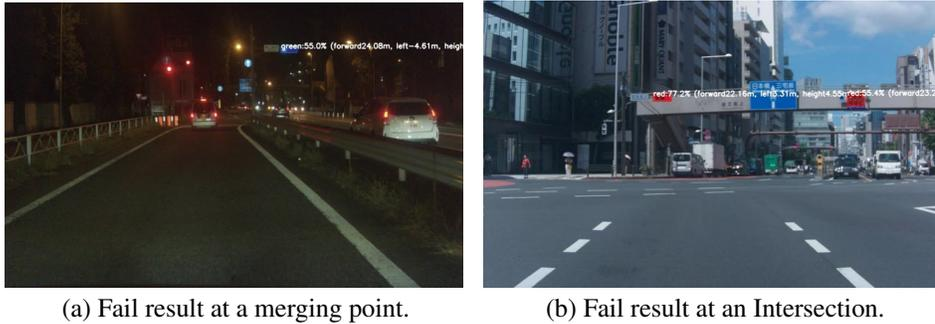
Figure 8: Examples of Traffic Signal Detection Failures.
