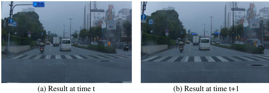
Figure 5: Detection results at times  $t$  and  $t+1$ , demonstrating the model’s capability to adjust focus from the nearer to the distant traffic signal as the scene changes.
