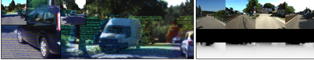
Figure 1: Samples from the real data. (Left) Zoomed in images on which 3D point clouds have been projected. The color of the points reflects the depth. We see three types of missing points: 1) the top part of the image is empty; 2) there are no points beyond 80m; 3) highly reflexive surfaces can produces missing or noisy acquisitions. We also see misalignment between the image and the point clouds, caused by either the change of viewpoints between the cameras and the LiDAR sensor, or by movement during the acquisition delay. (Right) RGB images with their corresponding pseudo-depth maps constructed from LiDAR point clouds.
