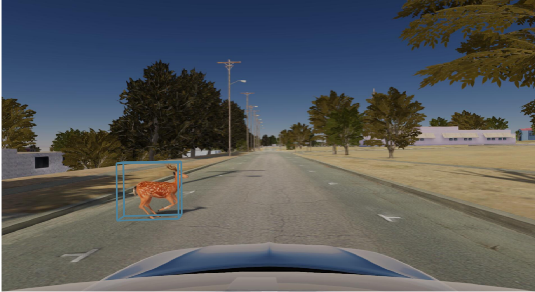
Figure 14: Camera Image for the scenario in Fig. 12. Blue bounding box is the ground truth detection. The camera fails to detect the deer crossing the road (misdetection failure).
