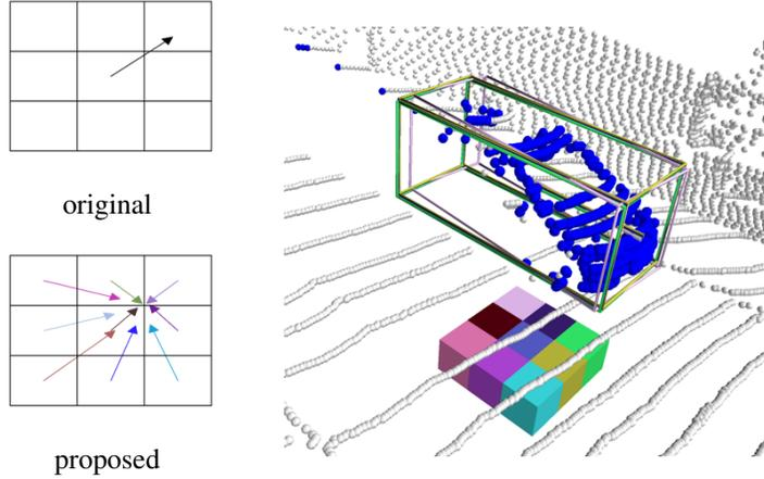
Figure 4: *Multi-cell Voting Scheme*. Rather than making a single hard prediction (top-left), our method produces multiple hypotheses by also making predictions in neighbouring cells of the feature map (bottom-left). A sample scene point cloud with the neighbouring cells and their corresponding predicted 3D bounding-boxes (right); colour of each bounding box encodes the source cell which produced it.
