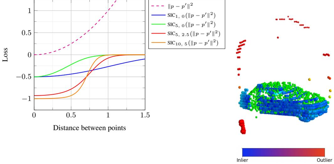
Figure 3: *Soft Inlier Count (SIC) loss*. Using L2 norm directly results in outlier points having a disproportionate influence on the loss minimising location. Different parametrisations of the SIC loss (left). An example matching of the 3D rigid model (green) to the detected object point cloud, with SIC loss value illustrated by the colour of each LiDAR point (right).
