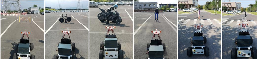
(a) Obstacle Avoidance: barrier, bicycle, motorcycle, dummy, person, and chair-like robot (from left to right)
