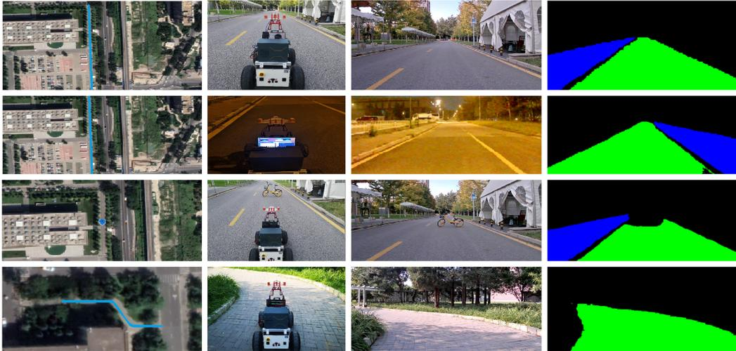
Figure 4: The bird’s eye views, actual scenarios, raw inputs, and semantic segmentation results (from left to right) for the tasks in Table 3 respectively.
