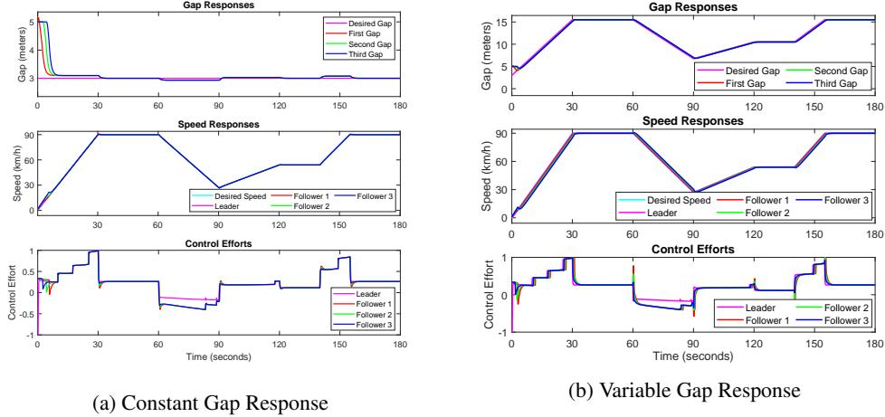
Figure 5: Gap, Speed and Control Effort of MPC for both constant and variable gap scenarios
