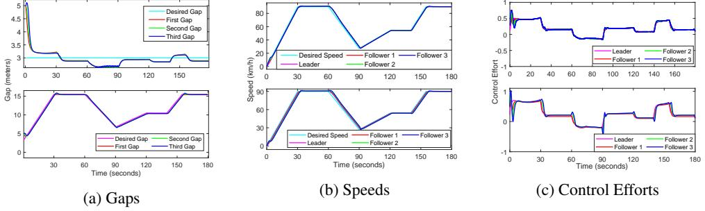
Figure 3: Response of Platooning Vehicles for the constant vs variable Gap scenarios, respectively
