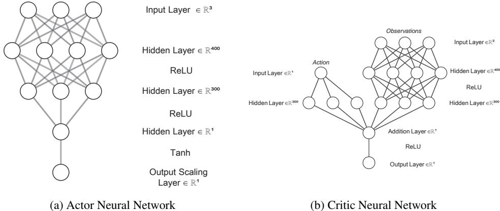
Figure 1: DDPG Neural Network Architecture
