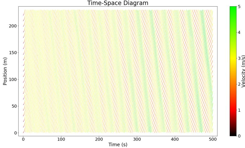
Figure 2: Formation of waves as 22 human drivers drive on the ring. Each line is the trajectory of a human driver and the red portions correspond to portions where vehicles have come to a near full stop. The alternating patterns of red and green indicate the formation of waves.
