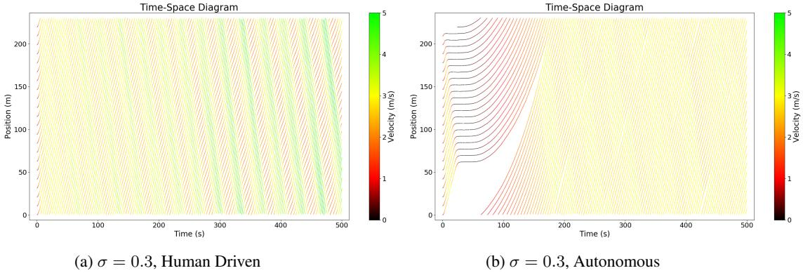
Figure 4: Time-space diagram of the system dynamics with a single controlled AV. On the left, the system is unstable without control while the waves are significantly smoothed with control on the right. Waves cannot be completely reduced due to the inherent noise in the system.
