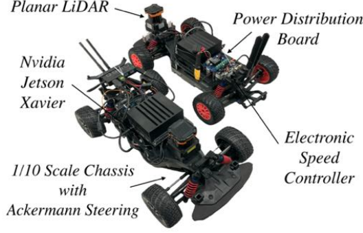
Figure 5: Components of the 1/10 Scale Vehicle
