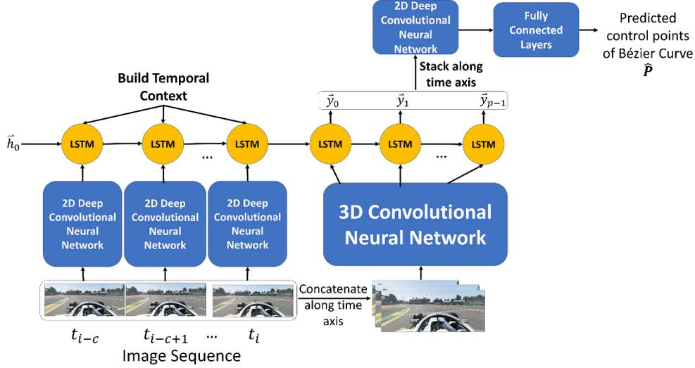
Figure 3: Architecture For The AdmiralNet Bézier Curve Predictor.
