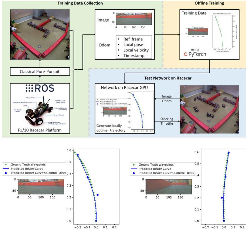
Figure 5: [Top]DeepRacing AI was implemented on a 1/10 autonomous racing testbed using ROS. [Bottom] The ground-truth waypoints and predicted B‘ezier Curve next to sample images from the testbed.
