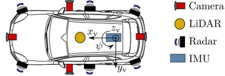
Figure 2: Sensor setup.
