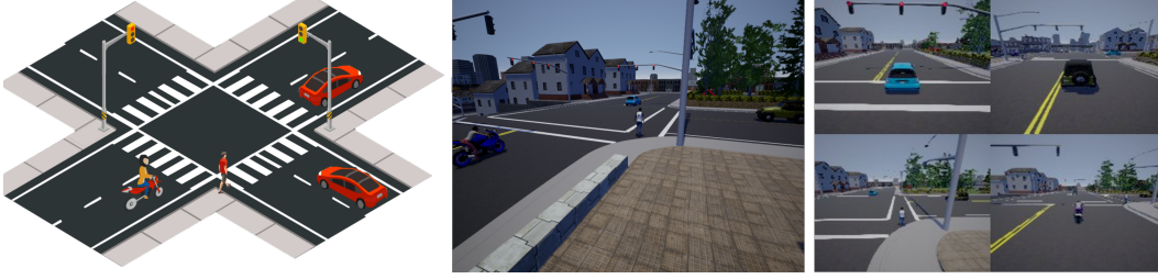
Figure 1: Figure shows a heterogeneous multi-agent learning environment created using MACAD-Gym. An overview of the scenario is shown in the left image. The middle image shows the simulated scenario and the right image shows tethered views of each agent’s observation
